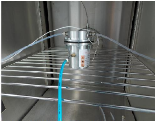
Sample inside Micro-SHED for emission test
